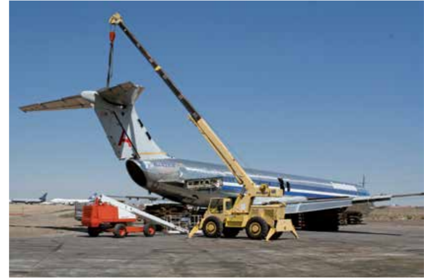
Left • The tail from N442AA (c/n 49468) being separated from the aft fuselage section. (All images Scroggins Aviation unless stated)
