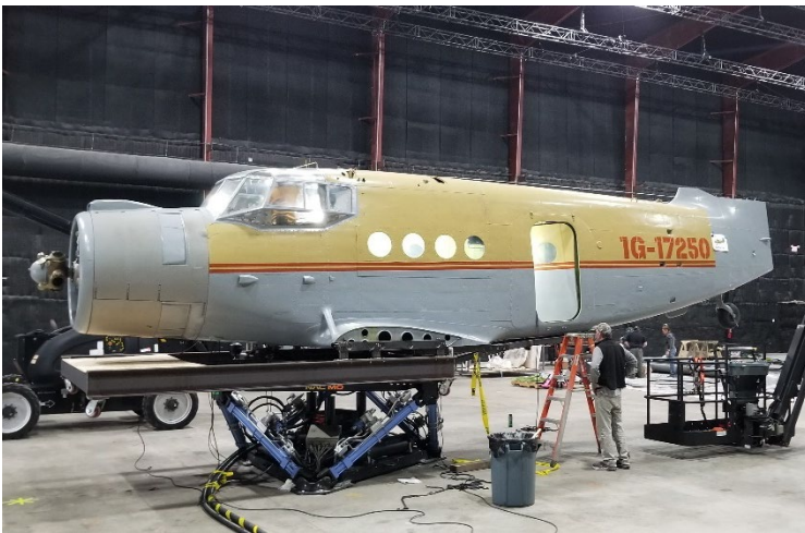
An-2 is shown mounted to on a steel frame structure for motion base work.
