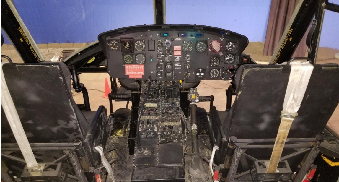
Some of the primary gauges work on command by operator. Cockpit windows and doors are wild.
