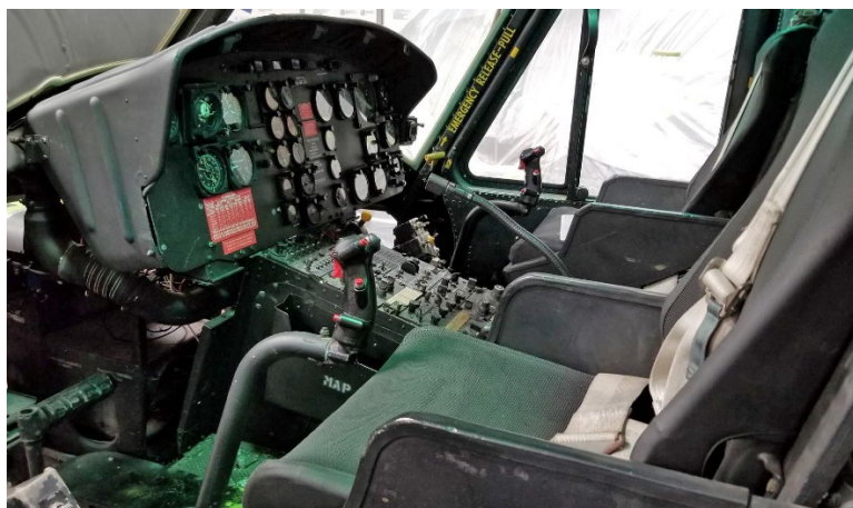
Cockpit panel works and lights up on command. (some smaller gauges are fixed)
