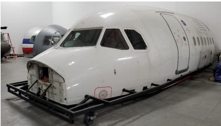
A320 shown with steel frame structure on the underside for motion base work
