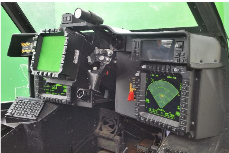
AH-64 is equipped with newer cockpit panels and gunner "TEDAC unit".
