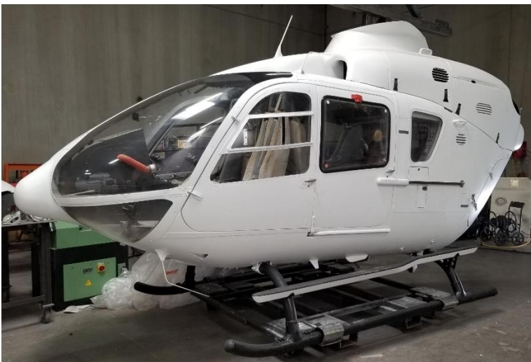
Shown with tail boom removed and on a shipping stand with casters.
