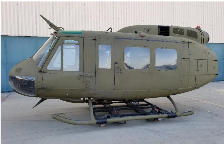
Mockup shown with tail boom and rotors not installed. It ships on a base w/ casters Cockpit main windows, doors and seats are wild for camera angles.
