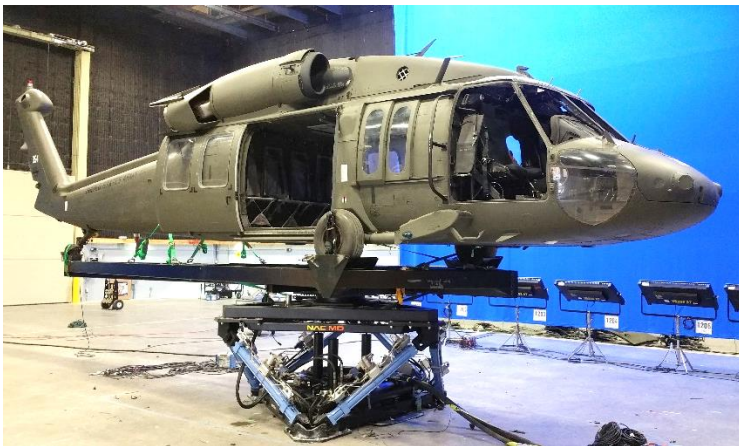
The real UH-60 is shown here mounted on a motion base (gimbal)
