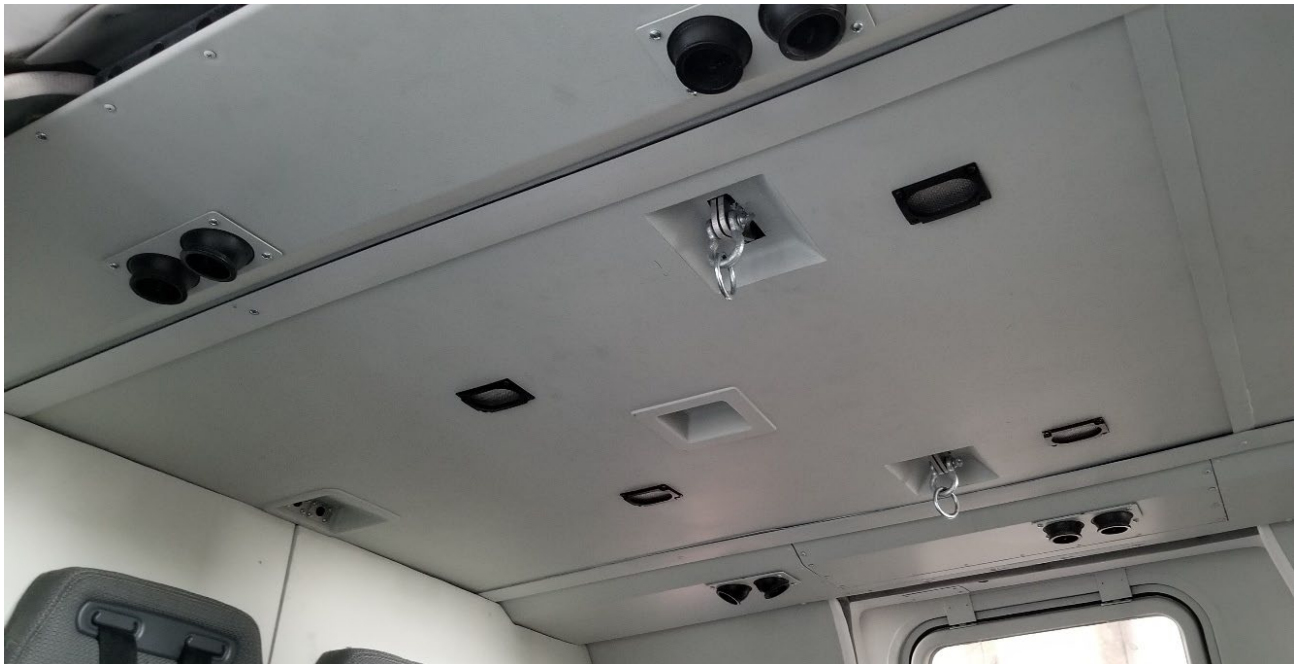
Main Cabin Ceiling with air vents, lighting and safety latches
