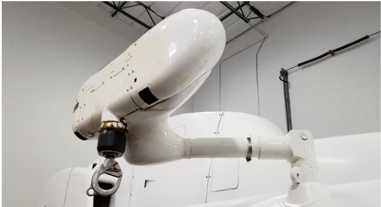
Hoist mounted to the right side of the S76 above the slider door.
