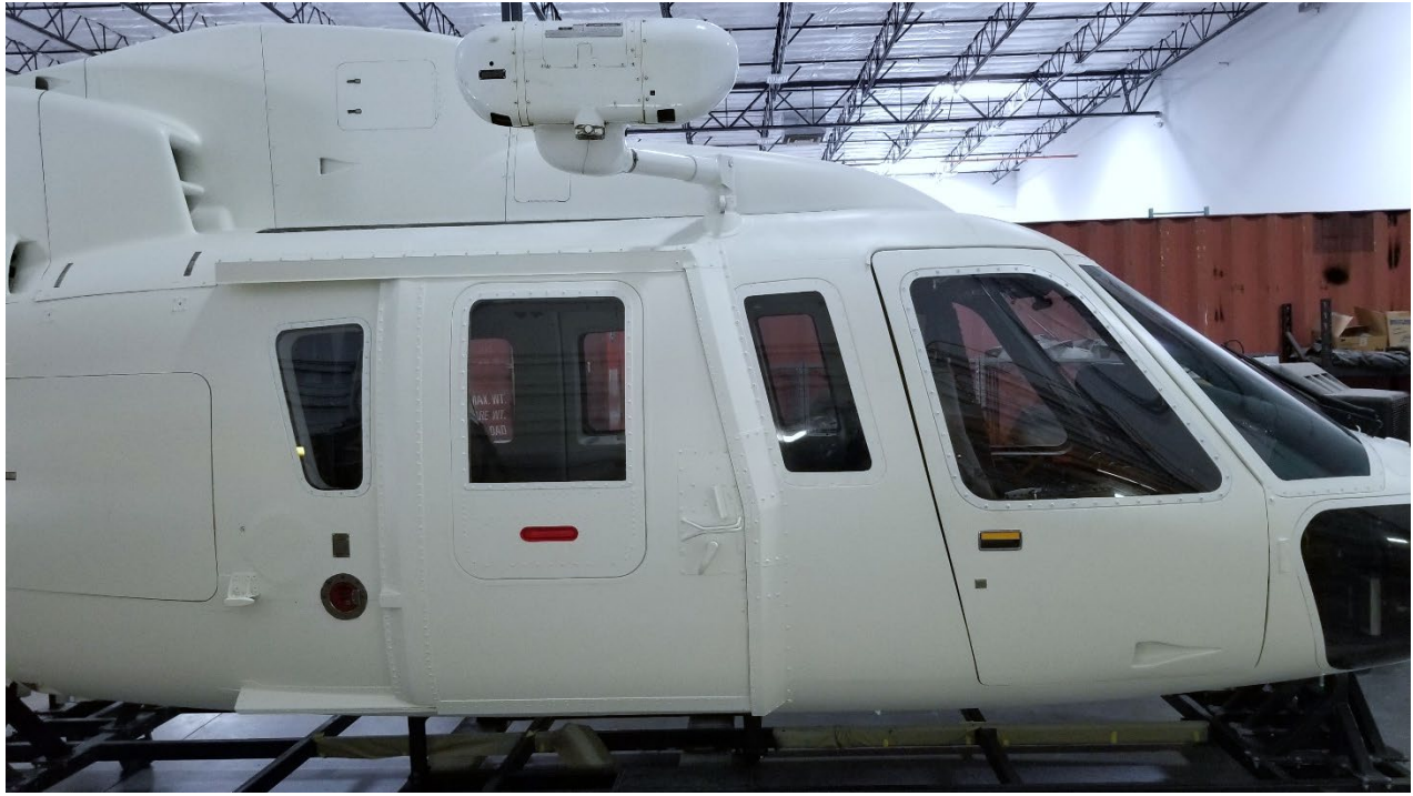
Rear cabin sliding door option with hoist located above the door frame.
