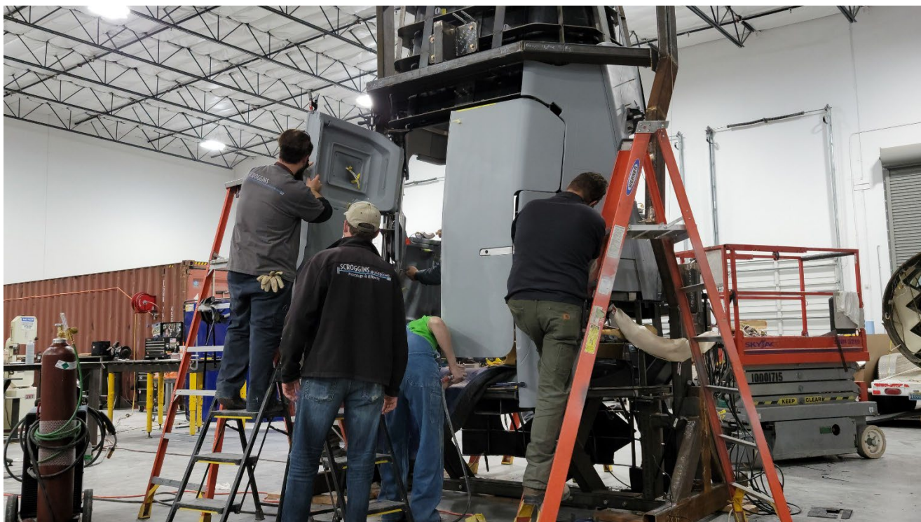
The Scroggins team works at assembling the escape vessel by attaching the plastic-formed panels and adding the control boxes to the inner walls. (Scroggins)
