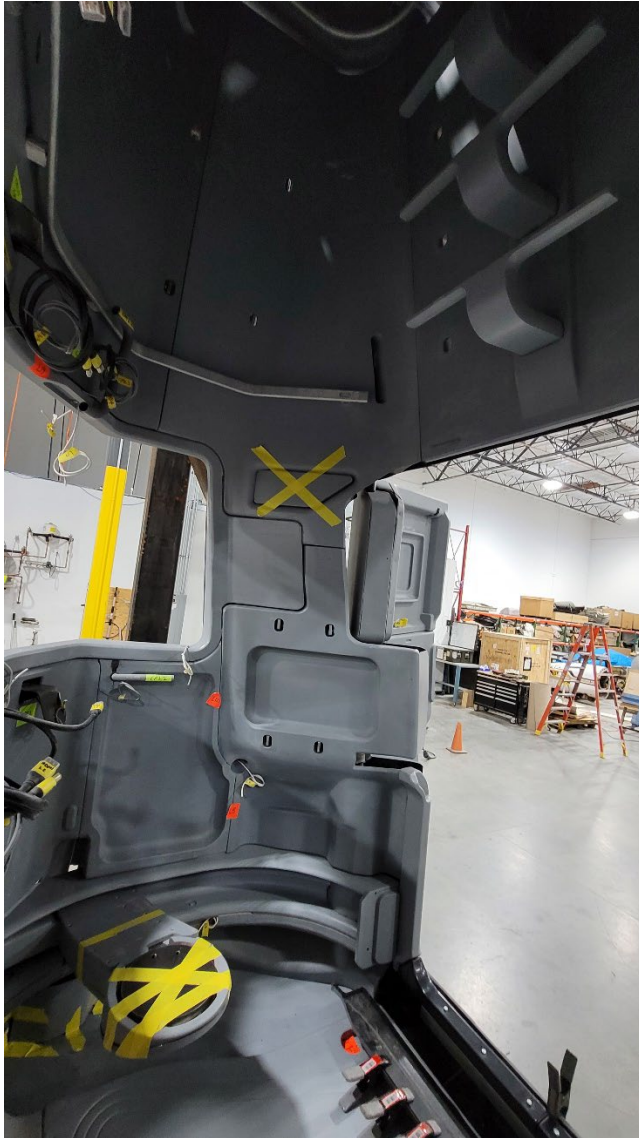
Interior of the escape vessel shows plastic panels in place, painted in primer and ready for color. Electrical wiring was run to key locations for monitors and lighting. (Scroggins)
