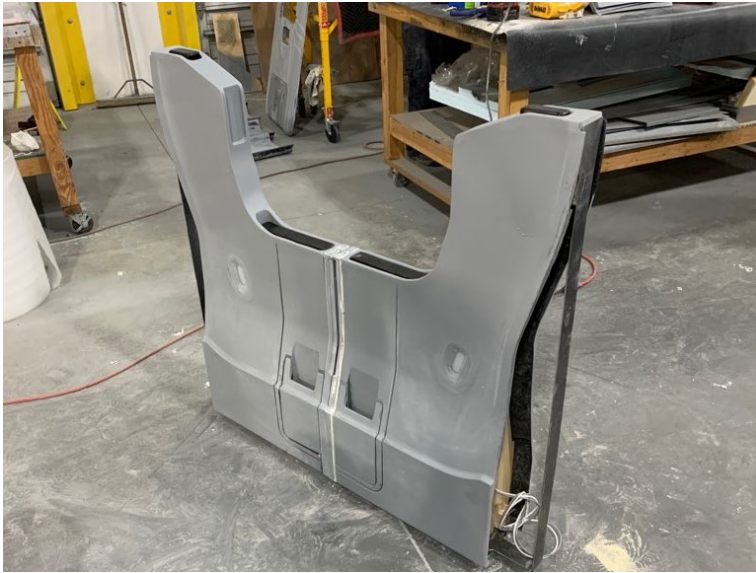
Build for the airlock doors, upper inner section, steel and wood inner structure with ABS vacuum-formed panels on the exterior. (Scroggins)
