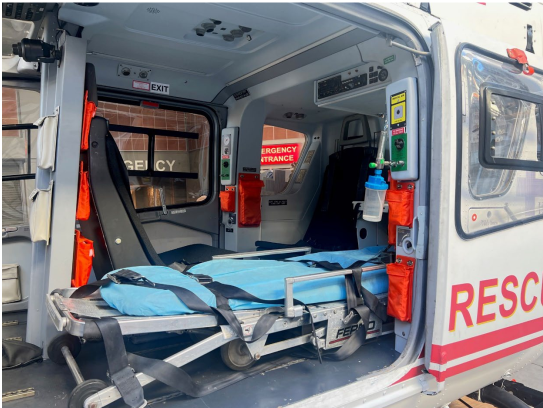
MedEvac cabin walls installed and dressed inside, rear clamshell doors open for stretcher.
